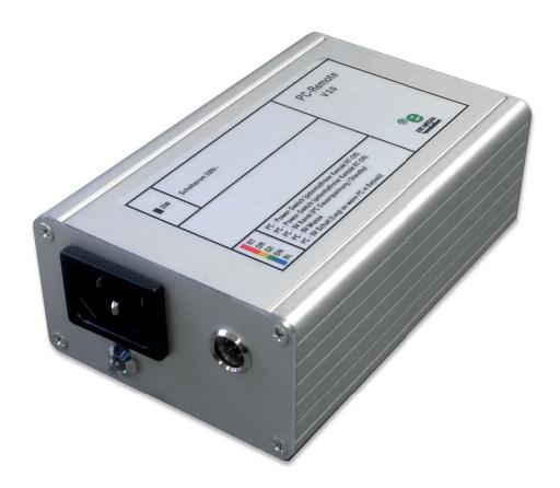
KLICK-KLACK ensures that PCs are started when switching on the switching current of an exhibition or installation and to carefully shut-down the PC when switching off the switching current in order to protect the data and hardware from damages.
